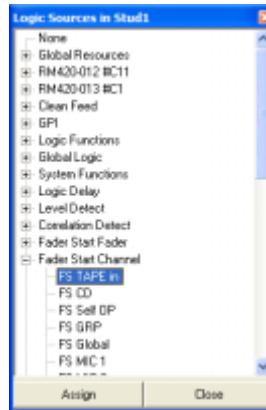
Figure 3-4: Logic Sources window. The name of the current Device is displayed in the title bar.
