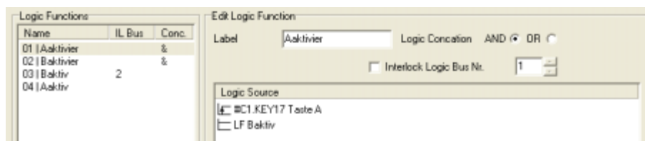
Figure 3-73: Interlock Example 4: Change of state with two keys, Logic Function 1.
