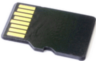
MicroSD card, side with pins.
