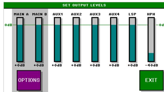
Touching a bar selects it and allows for level setting with the rotary. Turning the rotary will immediately change the level, no need to confirm the setting by pushing the rotary. In this way you can still set the outputs levels of the main outputs without the faders assigned to these outputs.
