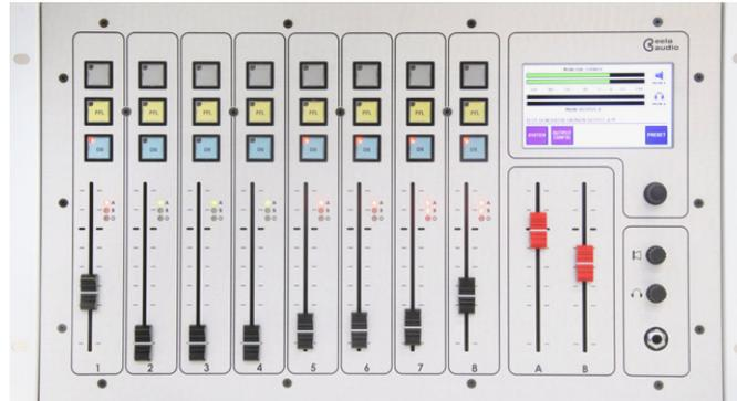
8 Channel input faders with 3 pushbuttons with LED:
