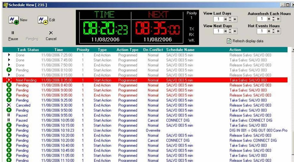
The screenshot shows the 'Schedule View [ 235 ]' window. At the top, there is a control panel with a 'New' button, an 'Edit' button, and a 'Priority 1' indicator. The central display shows the current time '08:20:23' in green and the next action time '08:35:00' in red. To the right of the time display are controls for 'View Last Days', 'View Next Days', 'Autorefresh Each Hours', and 'Hot Events Hours'. Below the control panel is a table of scheduled tasks.
