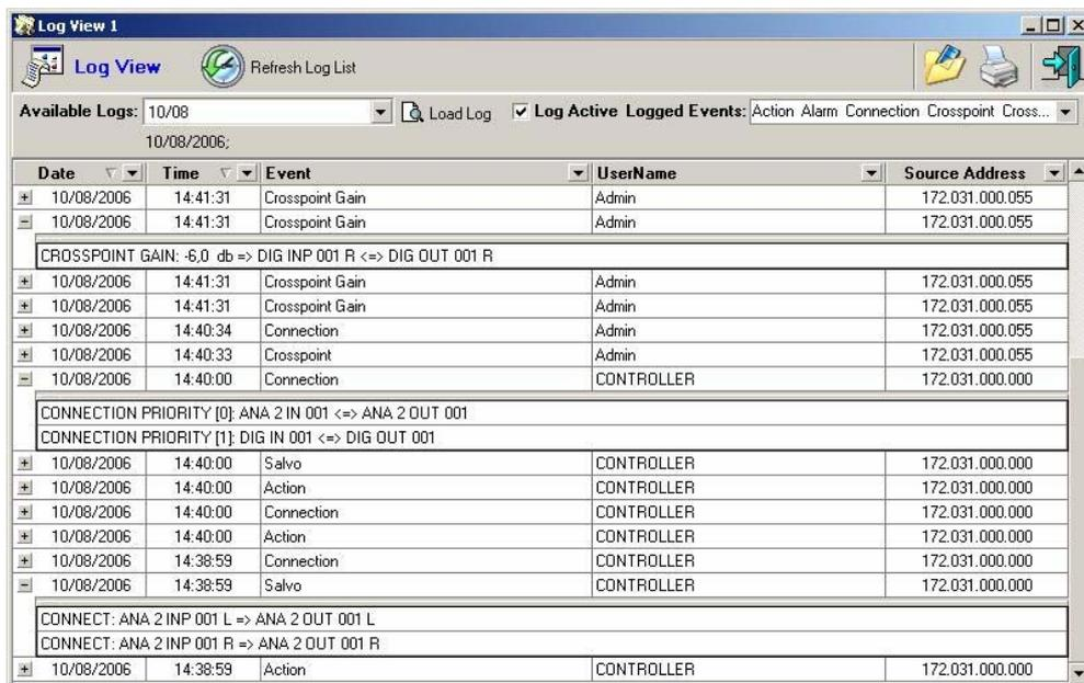
This table shows the date, time, event, user and location from which the action was executed (at the top right of this window the types of action that will be registered are shown, as previously defined by means of “BC 2000 D Matrix Setup” application). Associated with each event is a drop-down list that shows more specifically what the action performed consisted of.
