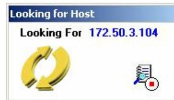
If the IP address configured in the software and the “Cluster IP“ are different, the following window appears where you can configure the right IP (it also appears if the IP is correct but the software can not connect with the active controller):
