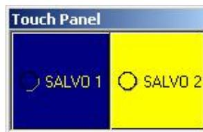
This touch panel window will have the characteristics implemented previously in your configuration as regards position, number and type of buttons and the actions they perform. The button may have a single operation associated (it will perform only a function when is pressed) or a double one (it will perform different functions depending on whether it is activated or deactivated).
