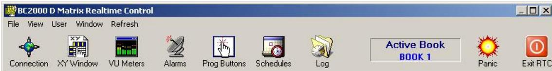
The buttons at the left side of the tool bar provide access to some of the options in the File menu: “New Connection View”, “New Logical XY View”, “New Vumeter View”, “New Alarm Status View”, “New Schedule View” and “New Log View”. You can find extended information about the features of these views in section 4.
