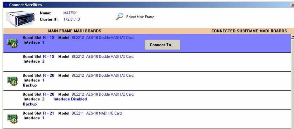
In the example, there are 3 MADI boards in the frame selected as main: one BC2212 board in slot 19, another one in slot 20 (configured in Backup mode, so the interface 2 appears as disabled) and one BC2211 in slot 21.
