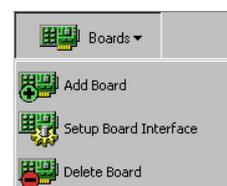
You can manually configure which boards are installed in the frame, one by one (by means of the “Add Board” button), or you can also accomplish this by using the “**Get Frame Board List**” button. This button gives you access to the following window, with information about the boards that are physically installed in the frame (on the left part), information that can be shifted over to the board lists displayed in the configuration software (on the right) by using “**Synchronize**” button:
