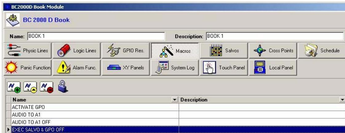
A macro is identified by a “Name” and a “Description”. In the “Working Groups” field, you can determine which working groups will have available the macro (input and output lines, salvos, etc.). You can also enable a request for user confirmation before executing the macro, by means of the “Ask Confirmation” box.
