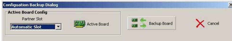
By pressing the **“Backup Board”** button, the selected board is configured as backup module of any other module of the same kind (the logical lines associated to a certain board are automatically associated to the backup module when there is some problem with the first one and it stops being active). You will be asked for a confirmation:
