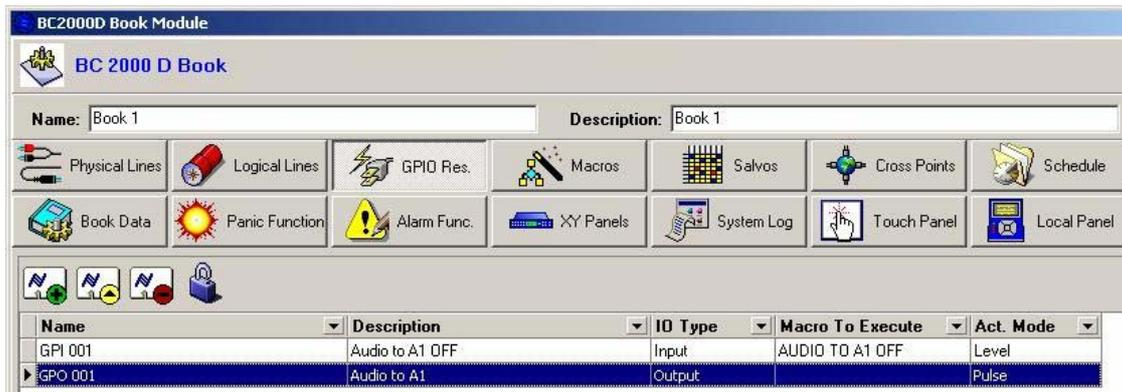
In this window you can define the programmable inputs and outputs that will be available in the system and the actions they will perform.
