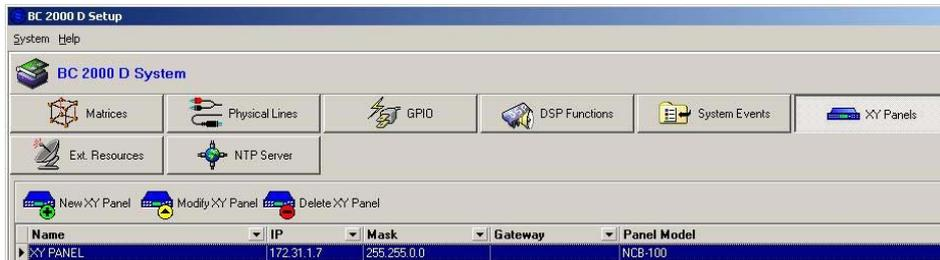
When “**New XY Panel**” is selected, a window opens where the name, model and IP address of the control panel are defined.
