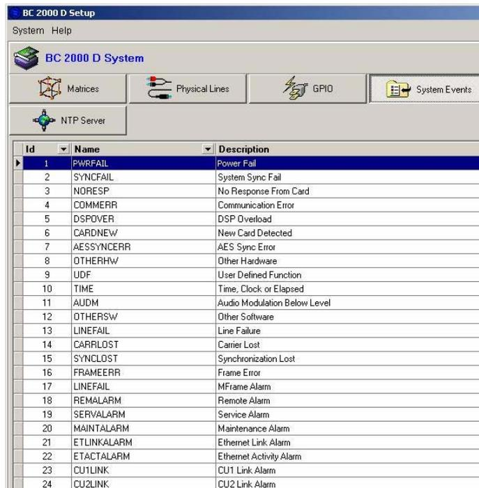
The screenshot shows the 'BC 2000 D Setup' software interface. At the top, there are navigation buttons for 'Matrices', 'Physical Lines', 'GPIO', and 'System Events'. Below these is a table listing system events with columns for 'Id', 'Name', and 'Description'.
